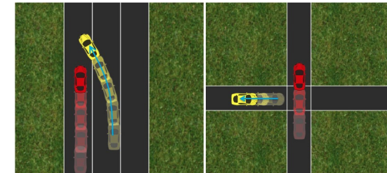
(a) Car merges ahead of human; anticipates human braking (b) Car backs up at 4way stop; anticipates human proceeding
